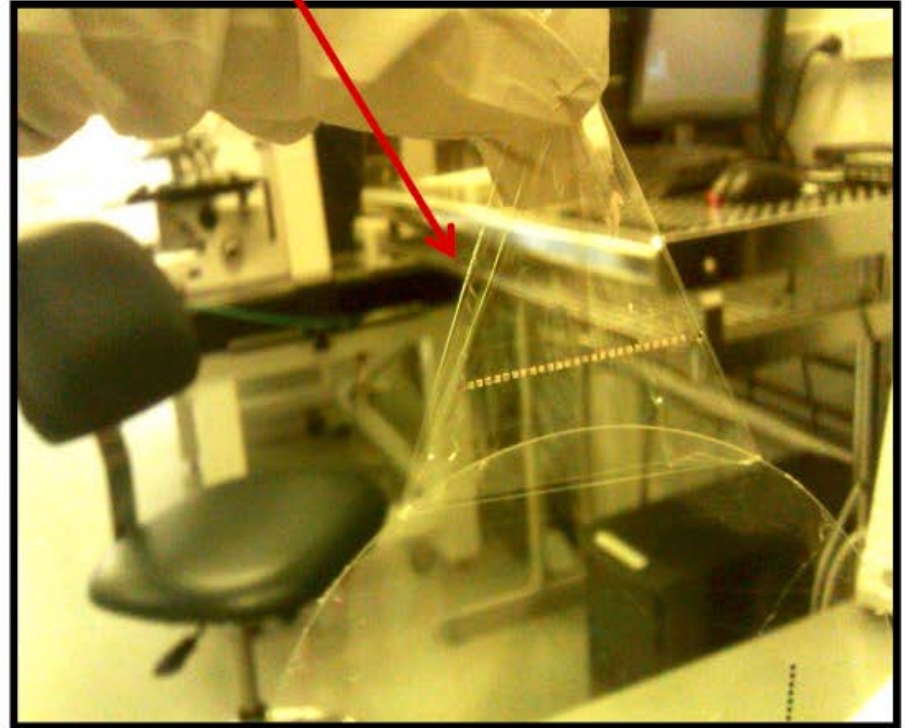
Parylene C – 4 \mu\text{m} thick
