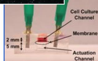
Mechanical Strain → Circular Pattern
