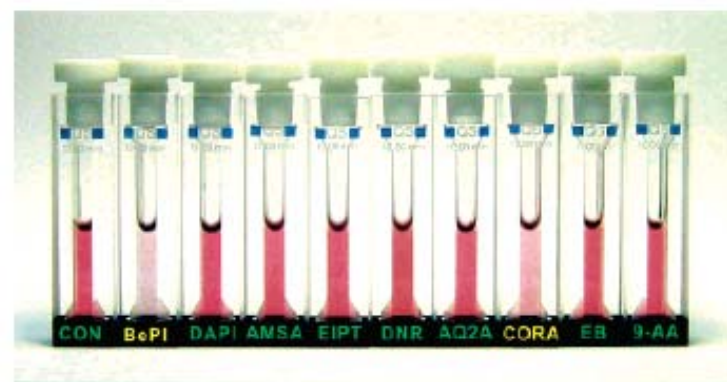
Figure 3. The color change of nanoassembly (NP-1, NP-2, and DNA-3) in the absence and presence of DNA binders at room temperature.
