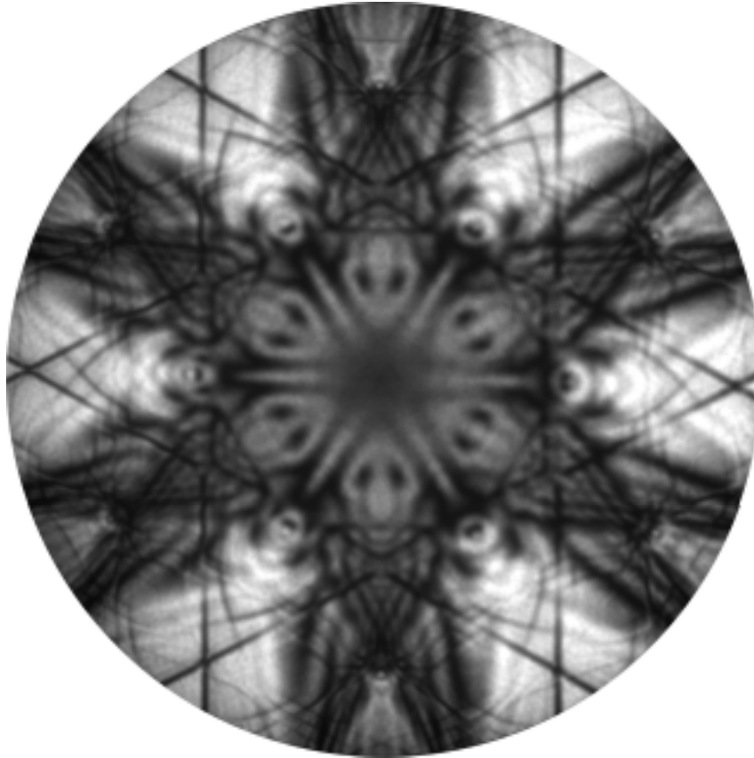
LACBED pattern along [111] of GaAs with buried InAs quantum dots
