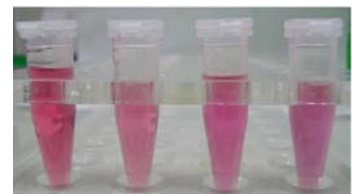
Gold nanoparticles, 20nm, 40nm, 60nm, 80nm in diameter P-K, Wei
