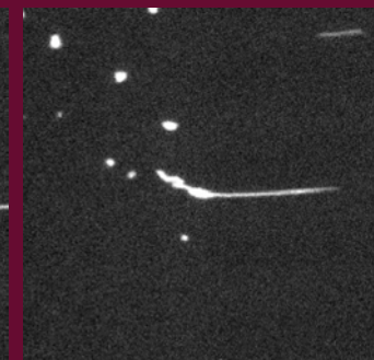
DNA strands going up the ramp in the interfaced area
